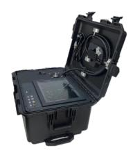
**FilmX** provides dual optical paths and excellent human-computer interface , which offers leading detection performance and easy operation . Its built-in balanced deuterium halide light source significantly improves the signal to noise ratio of the whole band .And the application of test optical path , reference optical path and dual optical path results in high accuracy.
