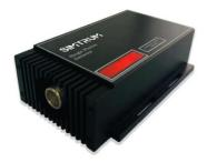
ST-APD works at as low as -20°C low temperature environment through internal cooling module to achieve the best signal-to-noise ratio. The refrigeration module is controlled by a highly efficient TEC and the control accuracy can reach  $\pm 0.2$ °C.
