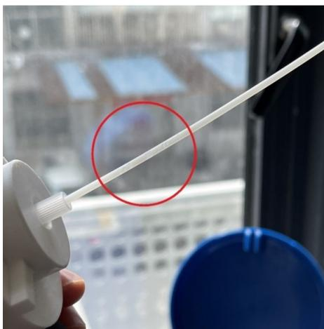
5.2. The liquid nitrogen tube will harden and become brittle under the influence of the refrigerating medium after normal operation. Do not swing vigorously, as it will cause rupture and damage. If you need to move the position, please wait until it returns to room temperature before operating
