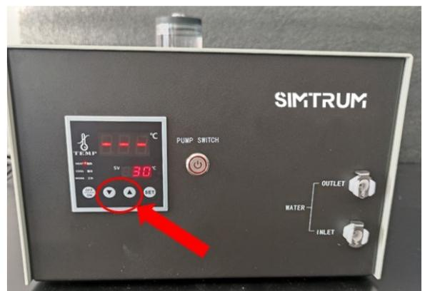
4.4 After setting the temperature, click SET again, and the circulating water system will perform the heating and cooling operation according to the set temperature.
