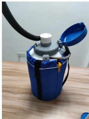
The silicone gas tube end of the liquid nitrogen converter is connected to the liquid nitrogen pipeline of the Optical Heating & Cryo Stages.
