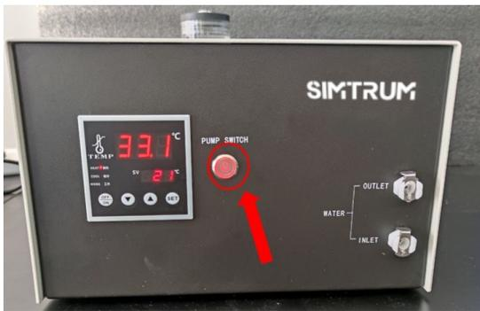
4.6 To close the circulating water system, it is necessary to turn off the switch on the operation panel, turn off the PUMP SWITCH button, and disconnect the power.
