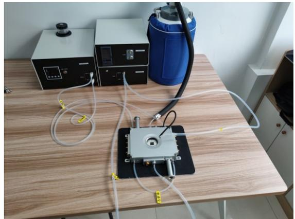
Note: The interface with the semiconductor circulating water system should be connected last to avoid water leakage during installation; there is no requirement for the order of entry and exit, and it should be ensured that the interface of the transfer pipe is on the same side of the table body.
