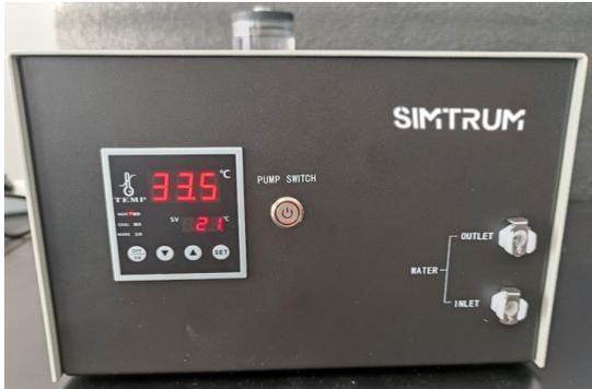
4.5 After turning on the PUMP SWITCH button, the pump will work, and the circulating water can flow into the pipeline.
