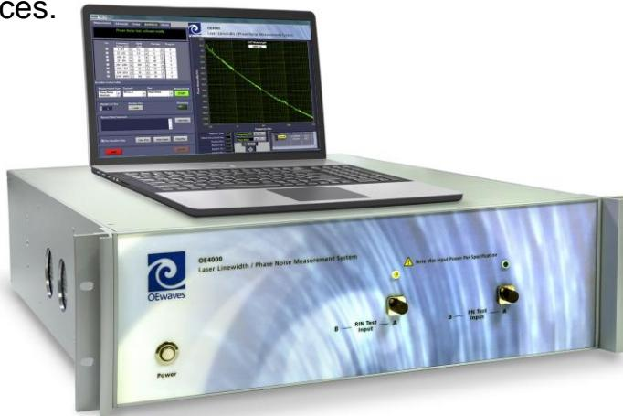
HI-Q® Optical TMS is capable of rapidly measuring laser phase noise and estimating its FWHM linewidth down to < 3 Hz without complex setup or reference lasers normally required to make such a narrow linewidth measurement.
